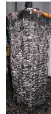
3 Hour FRR Column Test
