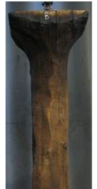
3 Hour FRR Column Test
